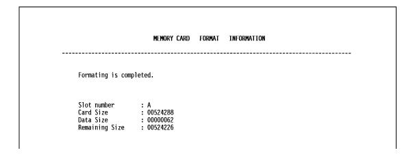
Slot number: Slot name for the memory card (only A is supported) Card size: The overall memory capacity of the card (in units of bytes)
